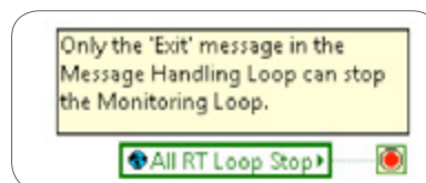
Figure 13.31. The RT Main VI stops if the user presses the Exit button on UI Main VI or if a critical error occurs within the RT Main VI.
