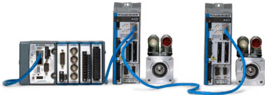
Figure 10.55. Any CompactRIO controller with two Ethernet ports can act as an EtherCAT master to control multiple daisy-chained AKD drives from the second Ethernet port.
