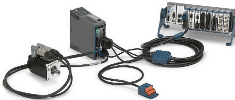
Figure 10.61. Directly connect cables between an NI 951x module and the analog AKD servo drive.
