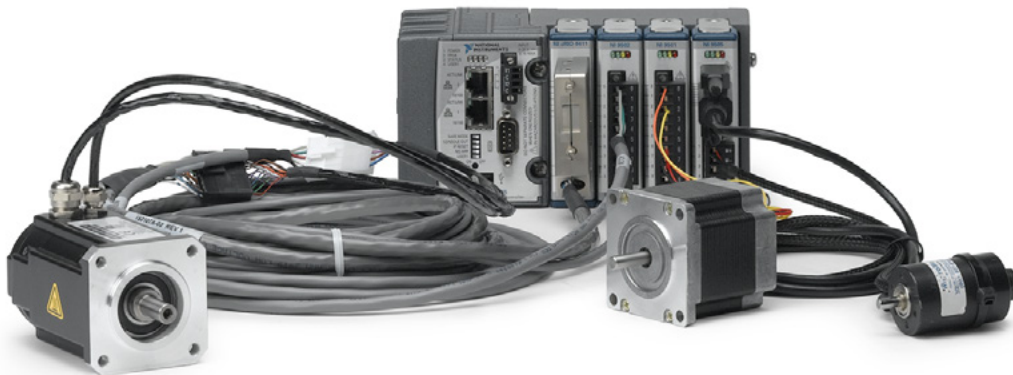
Figure 10.63. All that you need to run this system is an external power supply. An NI 9502 and NI 9411 are connected to the AKM brushless servo motor (left). An NI 9503 is connected to the stepper motor (center), and an NI 9505 is connected to the brushed DC motor (right). You can control all three motor types and organize them in different combinations from the same CompactRIO chassis.
